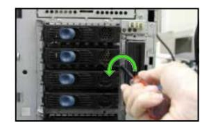
2. Carefully pull out the drive from the chassis until you see the cables connected to the drive.
